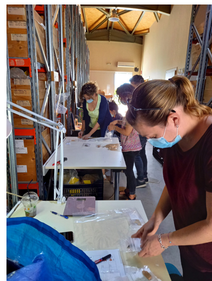
Below: Hundreds of briquettes prepared with clays collected from the wider Corinth and Sikyon area to assess their raw material physical properties
